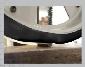
No-till fields can be rough on tires. Vegitation stalks and jagged rocks can make for a bumpy ride for your seeder/drill. AgriTraxx® AirCore™ acts like an additional shock absorber, conforming to debris & helping to maintain consistent seed depth. This also prevents the gauge tire from compacting the soil and promotes seed development.
